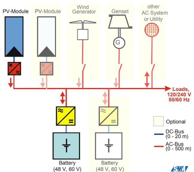
**Figure 1:** Comparison of mixed DC-and AC-coupled and pure AC-coupled System concepts for PV-Hybrid system design
