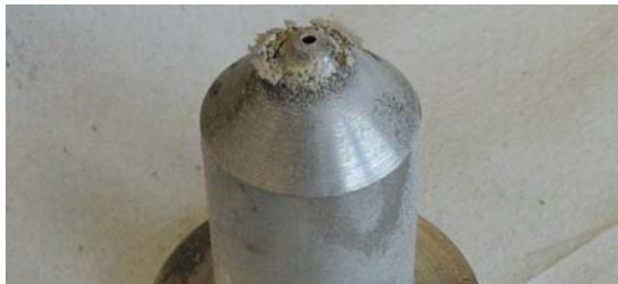
Fig.7: Deposits at jetpump nozzle using nitrogen as propellant
