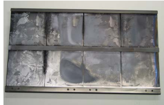
Fig. 8: Partially epitaxial deposition ( \text{H}_2 in the tube)
