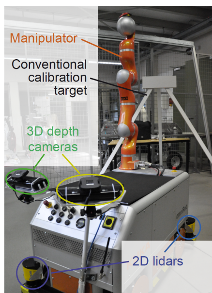
Figure 1: Placement of depth sensors on a mobile manipulator.
