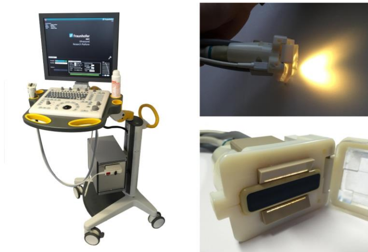
Figure 1. System overview and detail of transducer holder including custom made fibre bundle
