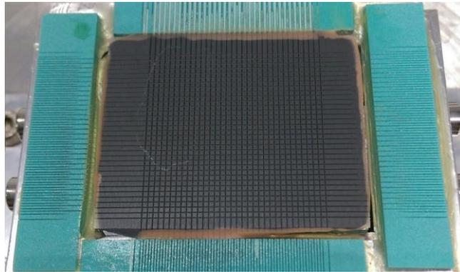
Fig. 6: First prototype of a 2D array with 1024 elements
