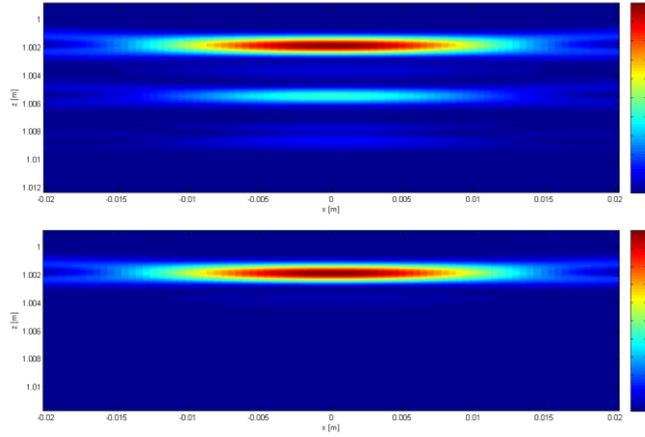
Fig. 2: Reconstructed point source without transmitting apodization (above) and with transmitting apodization (below)
