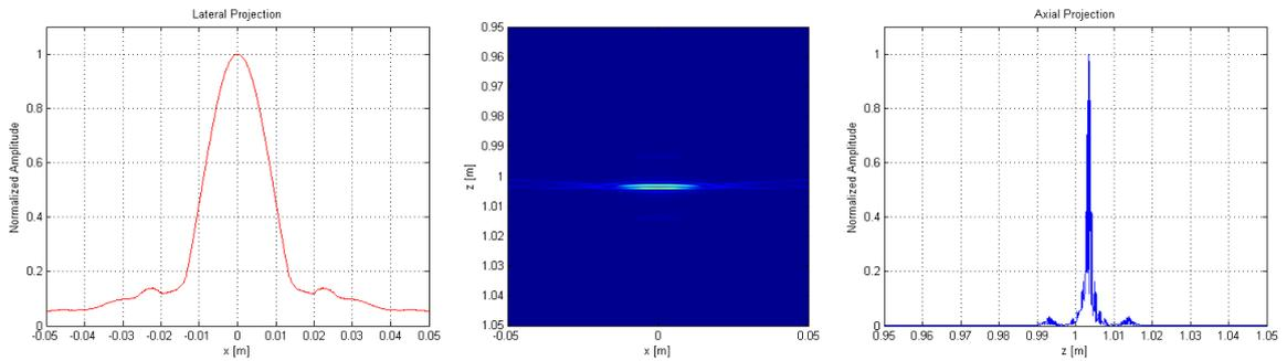
Fig. 3: Lateral and axial projection of the point spread function (PSF)
