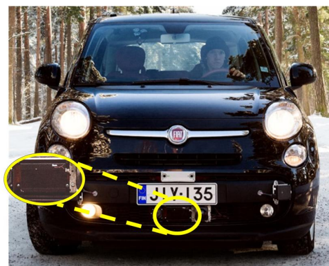
Figure 2. Laser scanner mounting location.
