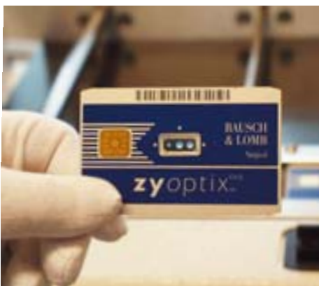
Card with three apertures for UV-laser ablation of the cornea of human eyes; small picture: detail.
