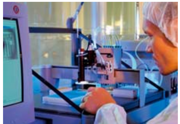
Dispensing bio molecules on electrical biochips in cleanroom environment.
