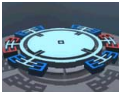
Figure 1: Model of an micromechanical angular- rate sensor for automotive applications.
