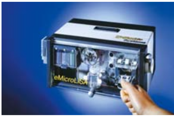
Figure 2: Insertion of the biochip packaged in a ChipStick.
