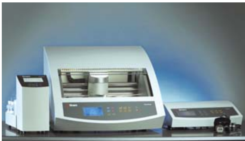
Figure 1: Overview of the Target Preparation System. Left side: Micropolishing System. Right side: Console for real-time alignment and measurement inside x-ray for hidden targets.
