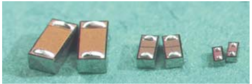
Figure 3: HPC components of different overall size, 0603 (left), 0402 (middle) and 0201 (right).
