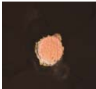
Figure 11: SnAgCu 0.5 – strong dissolution 1000x.
