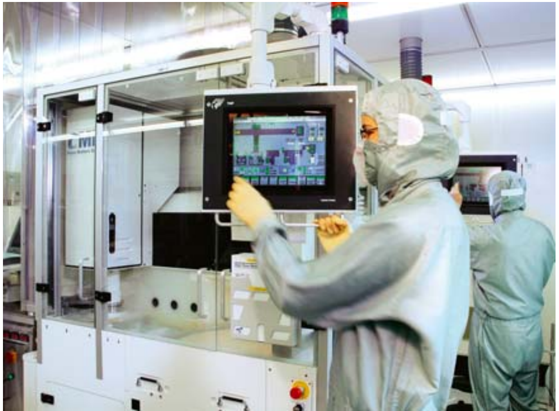
Peter Wolters PM 200 CMP™ cluster tool for planarization of MEMS devices.
