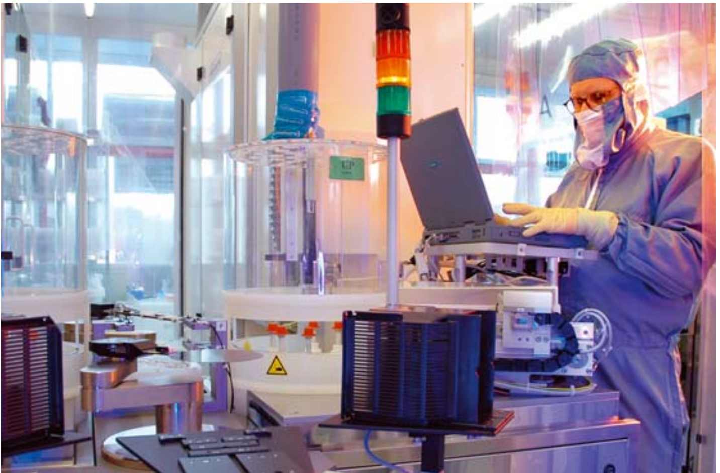
Cleaning module of PM 200 CMP™ cluster tool for MEMS applications.
