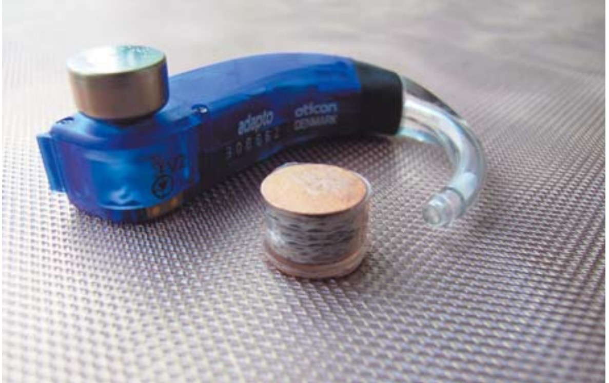
Figure 5: Prototype of a rechargeable battery in front of an external hearing aid.
