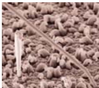
Figure 13: SEM image of a galvanic pure tin surface with different shapes of whiskers.
