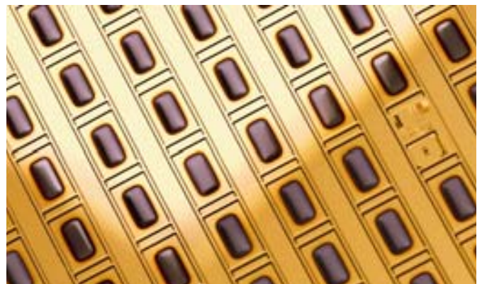
Cap wafer with individual getters for high vacuum sensor encapsulation on wafer level.
