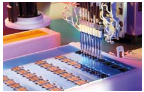
Figure 3: Detail of the Piezo-Plotter dispensing bio-molecules on the array positions of the electrical biochips.
