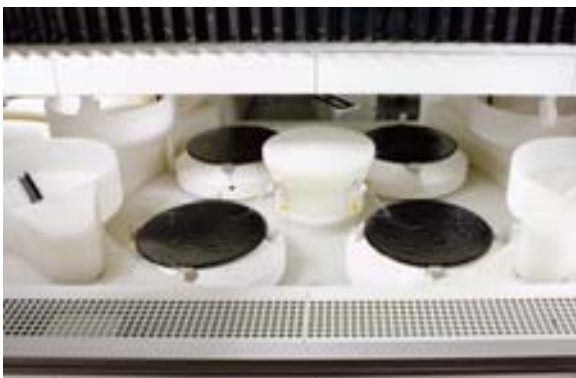
Wafer transfer station of Peter Wolters HFP™ CMP cluster tool.
