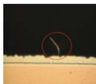
Figure 14: Microsection of tin layer with grown whisker (preparation plane measured with optical measuring station).
