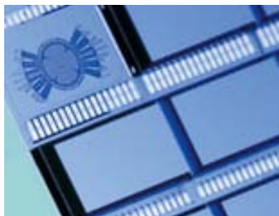
Figure 2: Sensor devices with and without Si-encapsulation on wafer level.
