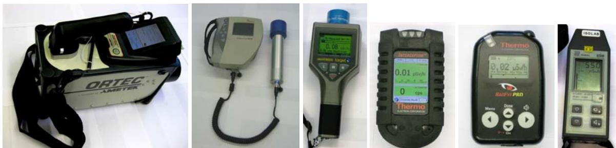
Figure 3: Detectors used for this study, from left to right: Micro Detective [4], InInspector 1000 [5], IdentiFINDER [6], Interceptor [7], RadEye PRD [8], FH40 G-L [9].
