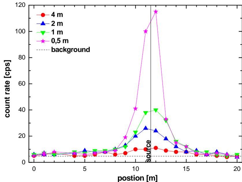
Figure 9: Localization of the Cf-252 source outdoors at different distances to the detector (count rate values taken from the static search mode in this case).
