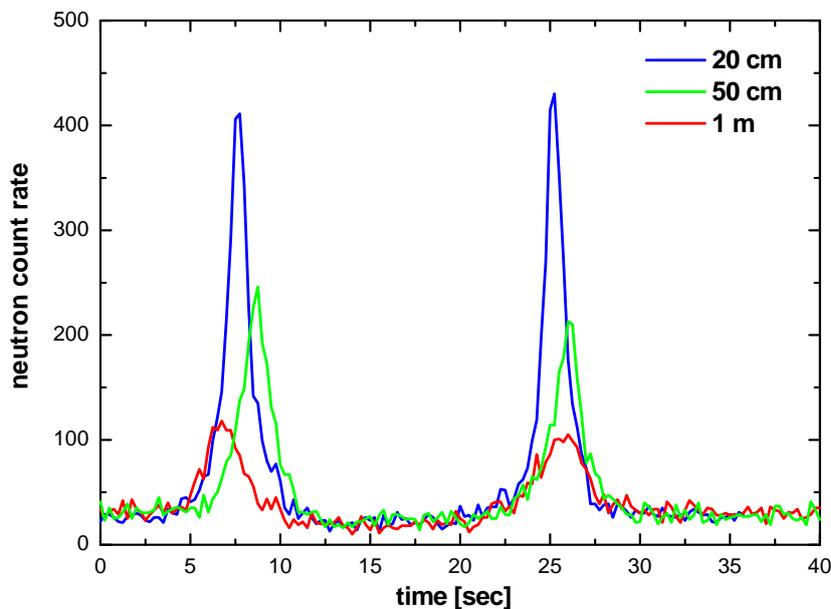
Figure 8: Localization of the Am/Li source in the lab at different distances.
