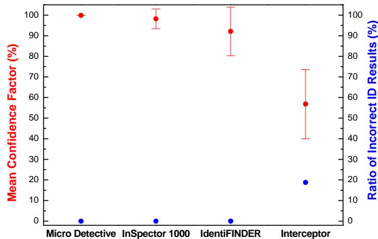
Figure 5: Comparison of mean confidence factors for all detectors featuring an identification mode (red dots) and false identification results (blue dots).
