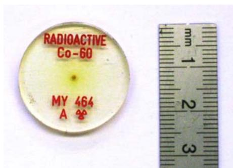
Figure 2: Co-60 source used for testing the search-qualification of detectors.
