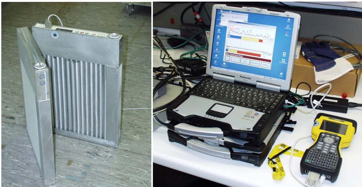
Figure 6: Fission Meter system with detector unit on the left and pocket PC / notebook computer for displaying the measured data on the right.
