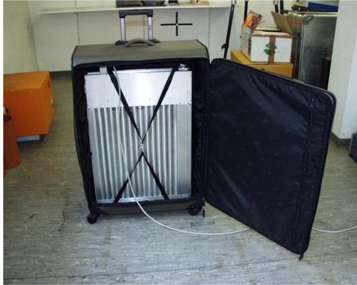
Figure 7: Detector unit strapped inside a trolley (setup for search experiments).
