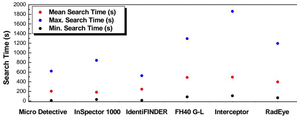
Figure 4: Comparison of mean, minimum, and maximum search times for all detectors and all groups of height. In two cases the source was not found at all; these data were not accounted for in the diagram.
