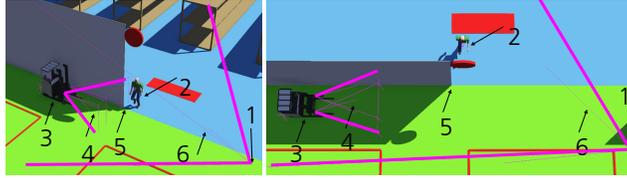
**Fig. 4.** Overview of the blind corner scenarios used in the simulation: (1) infrastructure camera, (2) human worker, (3) forklift, (4) forklift cameras field of view, (5) blind corner, (6) infrastructure camera field of view.
