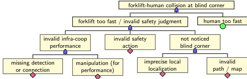
**Fig. 3.** Fault-tree of forklift-human collision for the functional architecture.
