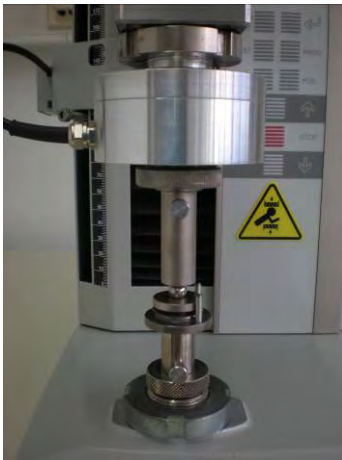
Figure 3: Ring on ring bending test for evaluating the mechanical strength of Silicon chips.
