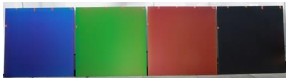
Figure 1: Full-area coating of module front glass cover [11]
