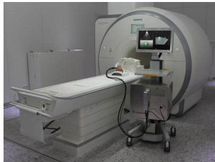
Fig. 1 MRI compatible ultrasound system for improved breast biopsy
