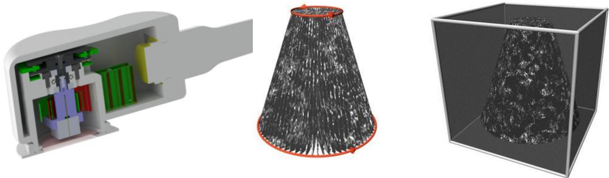
Fig. 2. (a) Section view of 8 MHz rotating ultrasound transducer; (b) acquired ultrasound slices; (c) calculated Volume
