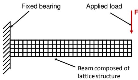
Figure 4: Bending loaded beam composed of lattice structures
