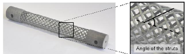
Figure 6: Torsion-loaded shaft composed of a helix-shaped lattice structure
