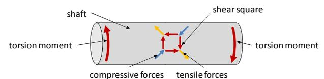
Figure 7: Shear square in a torsion loaded shaft (according to [15])
