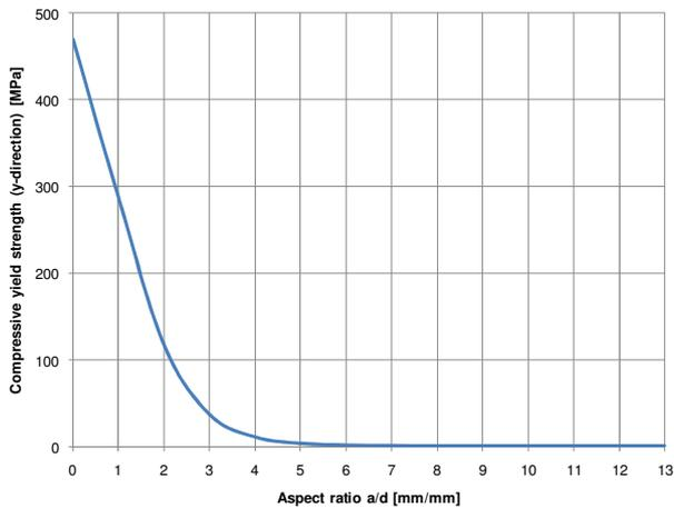
Figure 3 : Exemplary compressive yield strength types the ratio of their cell size  $a$  to strut diameter  $d$  (according to [3])
