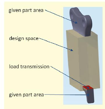
Figure 9: Pre-processing for the optimization procedure
