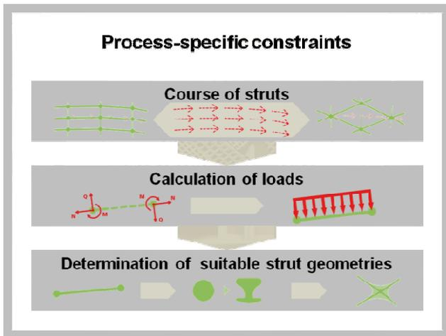
Figure 8: Procedure for flux of force dependent optimization of lattice structures
