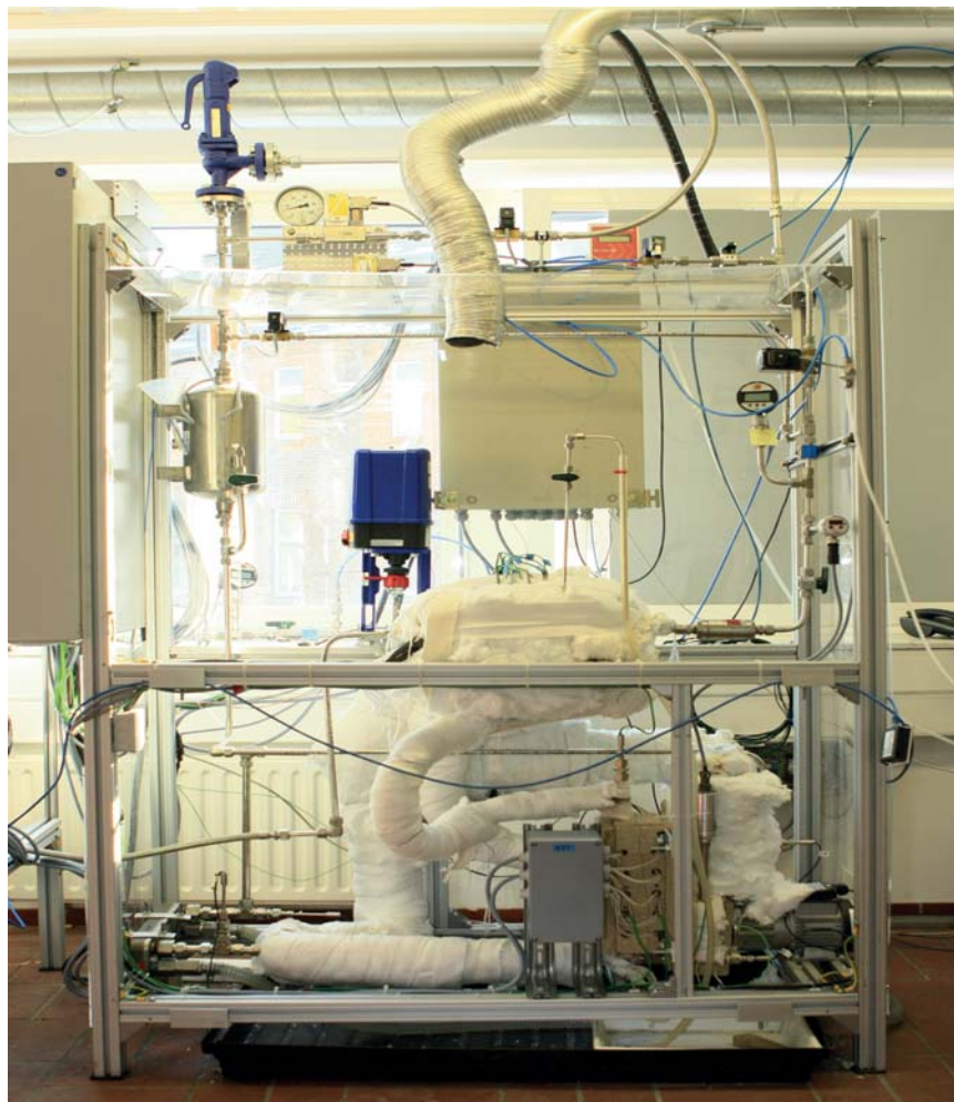
Figure 7.1: PtG lab-scale plant. Source: Fraunhofer IEE
