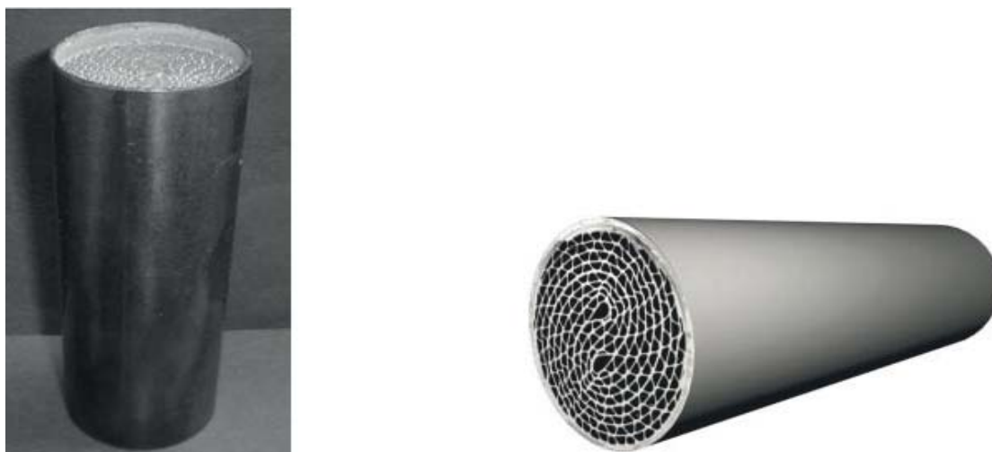
Figure 1.19: Honeycomb reactor developed at KIT
