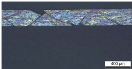
Figure 1. Edge cracks in a cold rolled aluminum sheet viewed in the direction of the roller axis.
