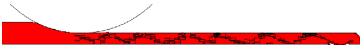
Figure 8. Zigzag pattern connected with edge cracking (from [15]). The elements with marked boundaries have failed.
