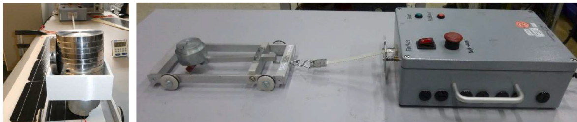
Fig. 4. Loaded metal blade which is dragged over the module frontside to simulate mechanical impact.
