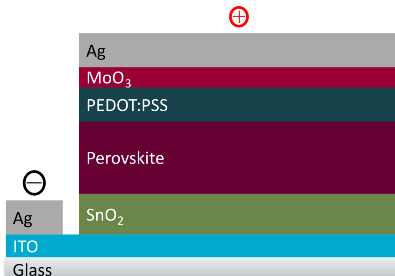
Figure 48: Schematic representation of n-i-p planar perovskite solar cells.
