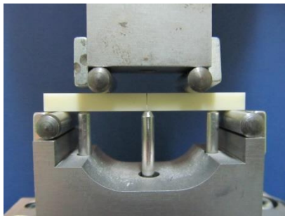
Fig. 2: Load configuration for the pre-crack formation under compression: The Chevron notch is on the upper (compression) side.
