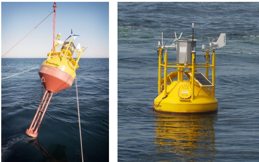
Figure 1 Prototypes #1 and #2 of Fraunhofer IWES Wind LiDAR Buoy – © Photographs: Fraunhofer IWES.
