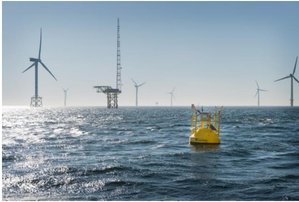
Figure 2 Setup and results of first offshore test (prototype #1) next to FINO1 met. mast used as reference.
