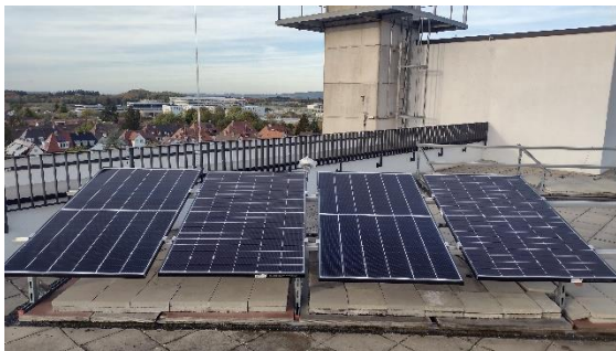
Figure 4: Four PV Modules, with one pair for each manufacturer M01 and M02, installed on a rooftop in Freiburg, Germany.
