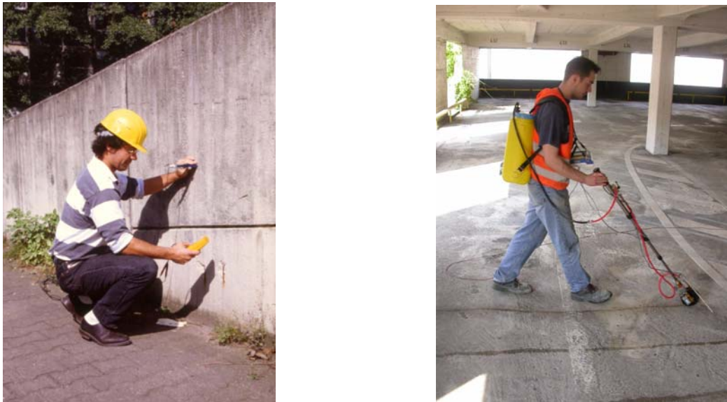
Figure 1: Potential Mapping using an handheld instrument point by point and a rolling wheel system
