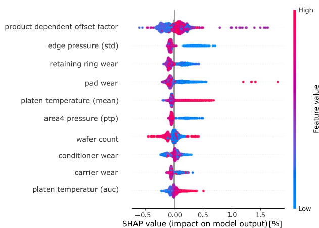
Fig. 13 Illustrates the SHAP summary plot for the 10 most important features of the final XGBoost model for predicting the WIWNU
