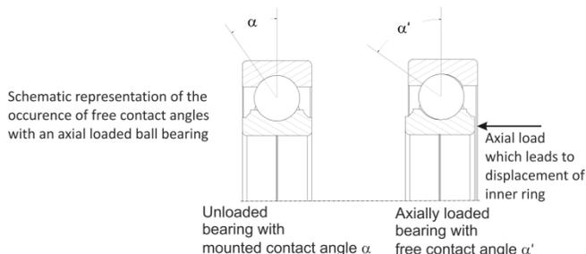
Figure 1: Schematic representation – Free contact angle
