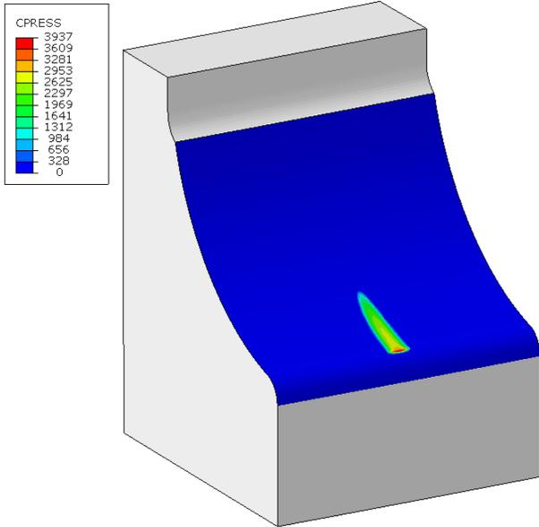
**Figure 23: Surface pressure in MPa during maximal Fres**
