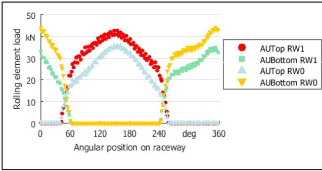
**Figure 8 Rolling element loads during OP 11**
