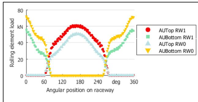
**Figure 7** Rolling element loads during OP 1
