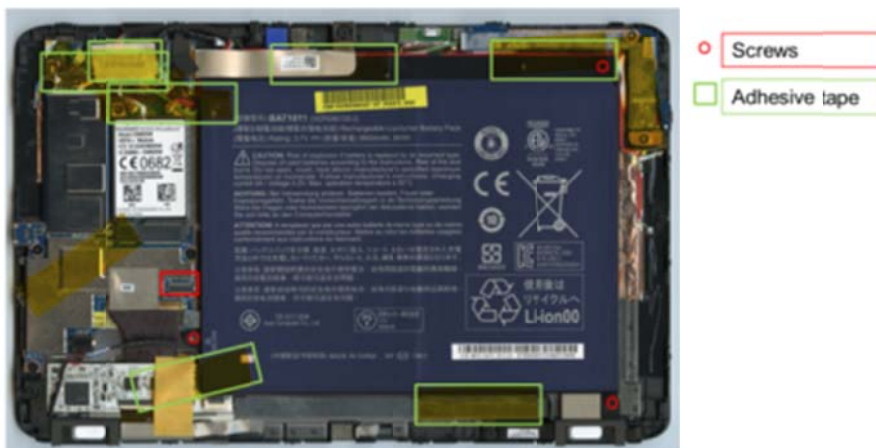
Figure 38: DUT_03 removal of battery
