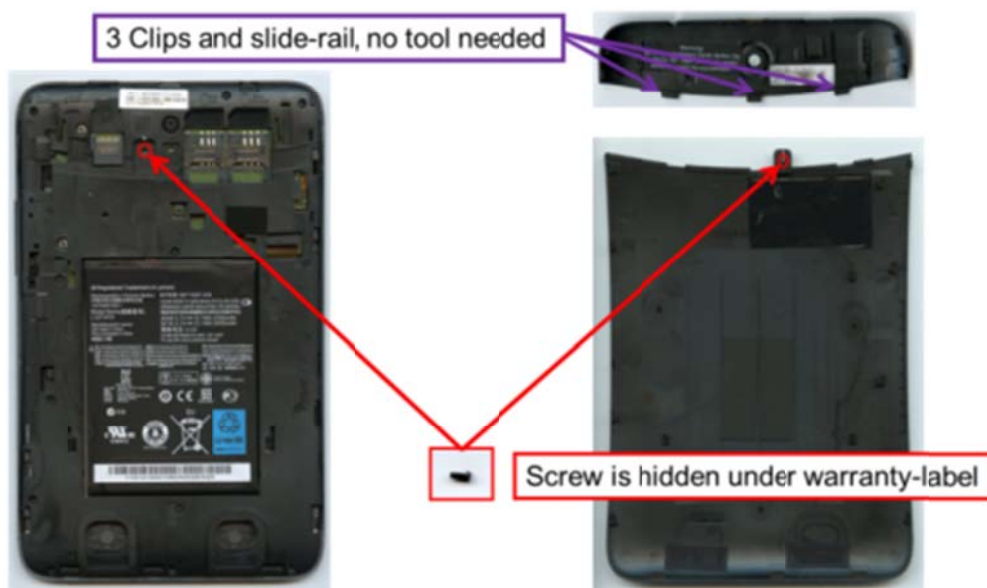
Figure 14: DUT_06 opening mechanism
