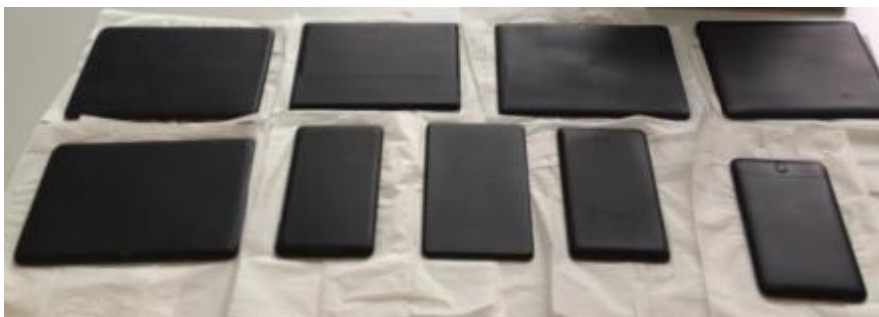
Figure 2: DUTs coated for thermography
