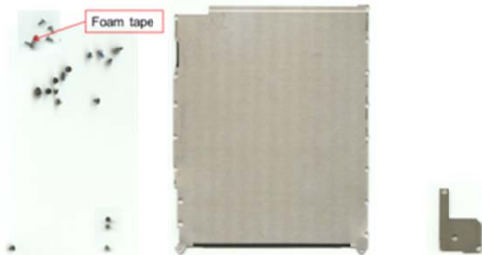
Figure 40: DUT_07 removal of metal shield
