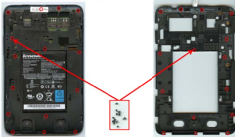
Figure 34: DUT_06 removing the inner frame
