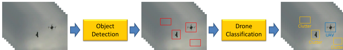
Figure 2. The established UAV detection pipeline. In the first detector stage flying objects are detected. A classifier in the second stage can then add semantics and reduce the number of false positive detections. The focus of this work is on the first stage. Note that missed detections from the first stage cannot readily be recovered in the second stage.
