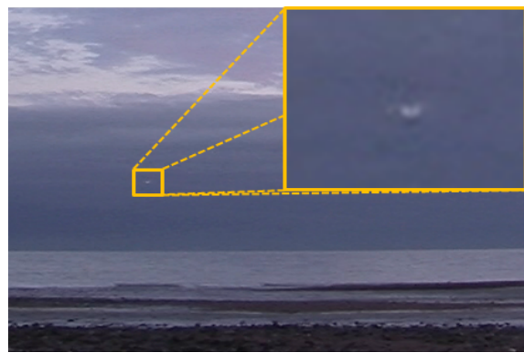
Figure 1. Detecting UAVs in image data poses several challenges such as very small object size, moving background, e.g., sea and clouds, varying illumination conditions, or weak contrast between the UAV and the background.
