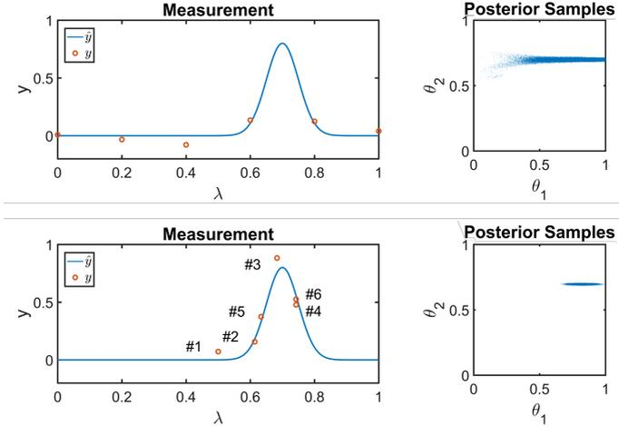
**Figure 3.2:** Comparison between equidistant measurement and adaptive measurement. First row: equidistant measurement and its corresponding posterior estimation. Second row: adaptive measurement and its corresponding posterior estimation.
