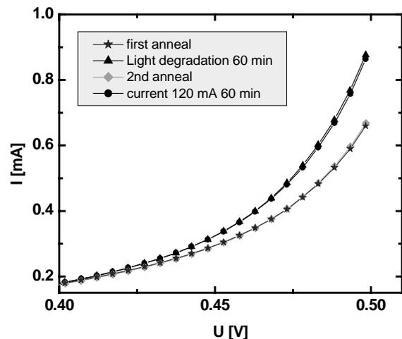
Fig. 1: Dark I-V characteristics of a CZ PERL solar cell after the first anneal, after 60 min. light degradation, after 2nd anneal, and after 60 min. current degradation
