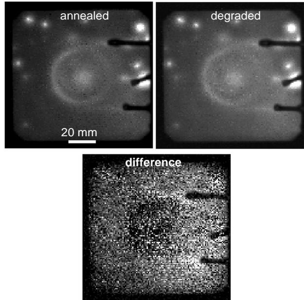
Fig. 6: Lock-in thermograms of the screen-printed cell before and after degradation (both scaled to 2 mK) and difference image (scaled to 0.2 mK)
