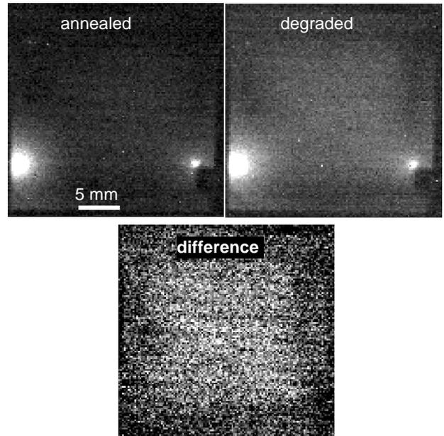
Fig. 4: Lock-in thermograms of the PERT cell before and after degradation (both scaled to 0.2 mK) and difference image (scaled to 0.05 mK)
