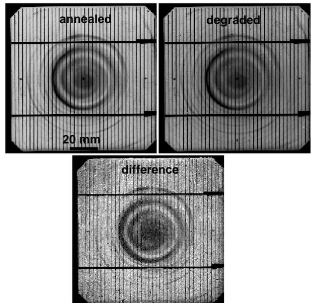
Fig. 7: LBIC images of the screen-printed cell before and after degradation (both in the same scaling) and difference image
