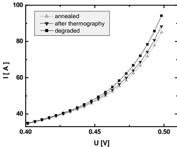
Fig. 5: Dark I-V characteristics of a 10\*10 cm<sup>2</sup> CZ solar cell after the anneal, lock-in thermography and after 120 min. current degradation
