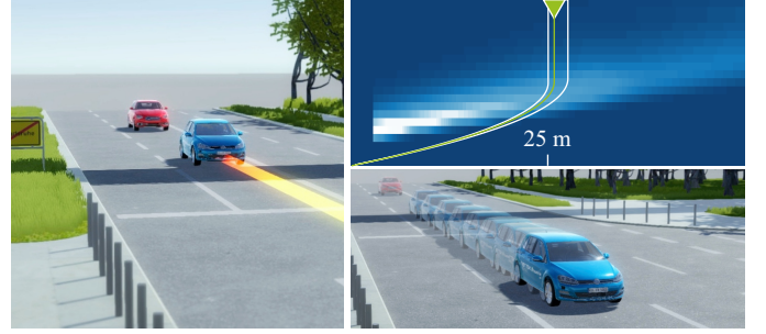
(b) In this inner city scenario (continued in the following frames), the ego vehicle is followed closely by another car. With a free straight path, a gentle deceleration minimizes the risk of a rear-end collision as above.
