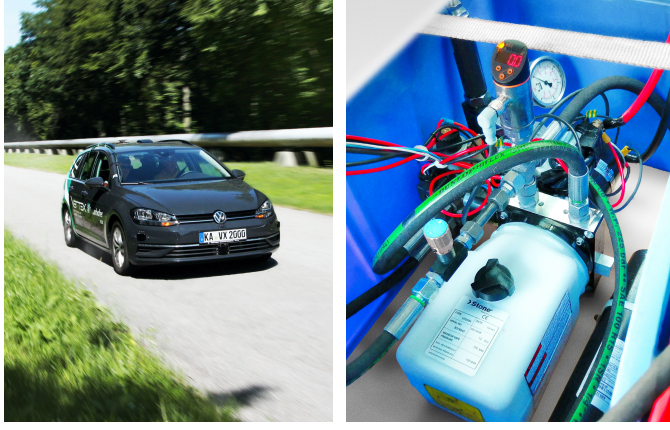
(a) Experiments for longitudinal accuracy with prototype installed in the VW Golf 7 Variant test vehicle. (b) Hydraulic / mechanical prototype in the back of the vehicle.
