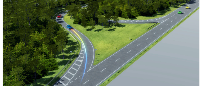
(a) In a system failure of the blue car, traveling at about 60 km/h (35 mph), a full braking maneuver would risk a rear-end collision with the following car, possibly also a loss of traction, depending on road conditions. If the steering wheel is locked to maintain the current curvature (indicated rainbow line), the vehicle can safely decelerate more gently without entering the highway.
