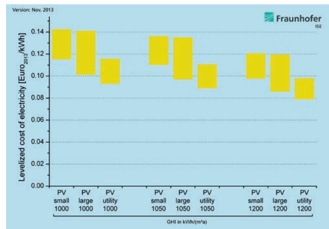
Figure 8: LCOE of PV plants in Germany based on system type and irradiation (GHI in kWh/(m²a)) in 2013.
