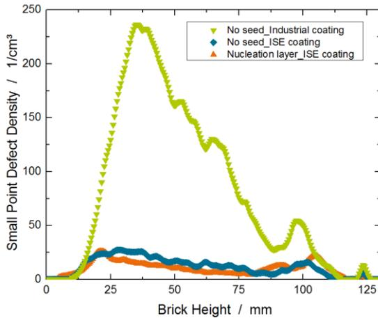
**Figure 2:** Small Point Defect Density over brick height for three different bricks. There are 10 times more small inclusions in the brick grown in the crucible with a standard industrial coating than the ones with the ISE coating.
