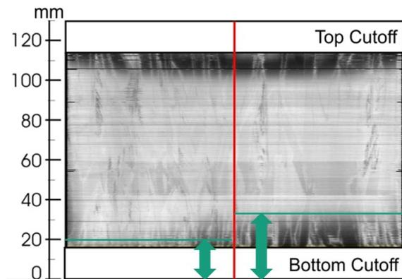
**Figure 6:** Virtual cross section through the brick using all wafer PL-images. In the bottom part, the different widths of the impurity indiffusion zones for the two seeding layers are indicated. The height was calculated using a PL-intensity threshold.
