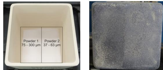
**Figure 1:** Experimental setup with two different grain size distributions on every half of the G1-sized crucible bottom (75 - 300 μm left and 37 - 63 μm right) and the bottom of the resulting Si-ingot.
