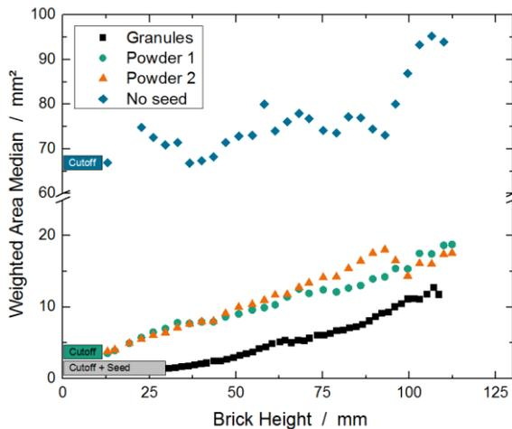
**Figure 4:** Weighted area median over brick height for the three bricks. The grain structure in the SiO<sub>2</sub>-seeded brick shows a similar evolution like the one grown on granules, being about 2 mm<sup>2</sup> bigger in size.
