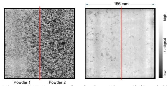
**Figure 5:** PL images of wafer from 10 mm (left) and 60 mm (right) ingot height. Different seed grain sizes were placed on each half. There is a clear difference in impurity indiffusion area and dislocation density for both sides.
