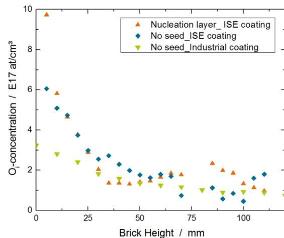
**Figure 9:** O<sub>i</sub>-concentration over brick height; The distribution is comparable, only in the first centimeters the value is slightly higher in the sample with SiO<sub>2</sub>-seed.
