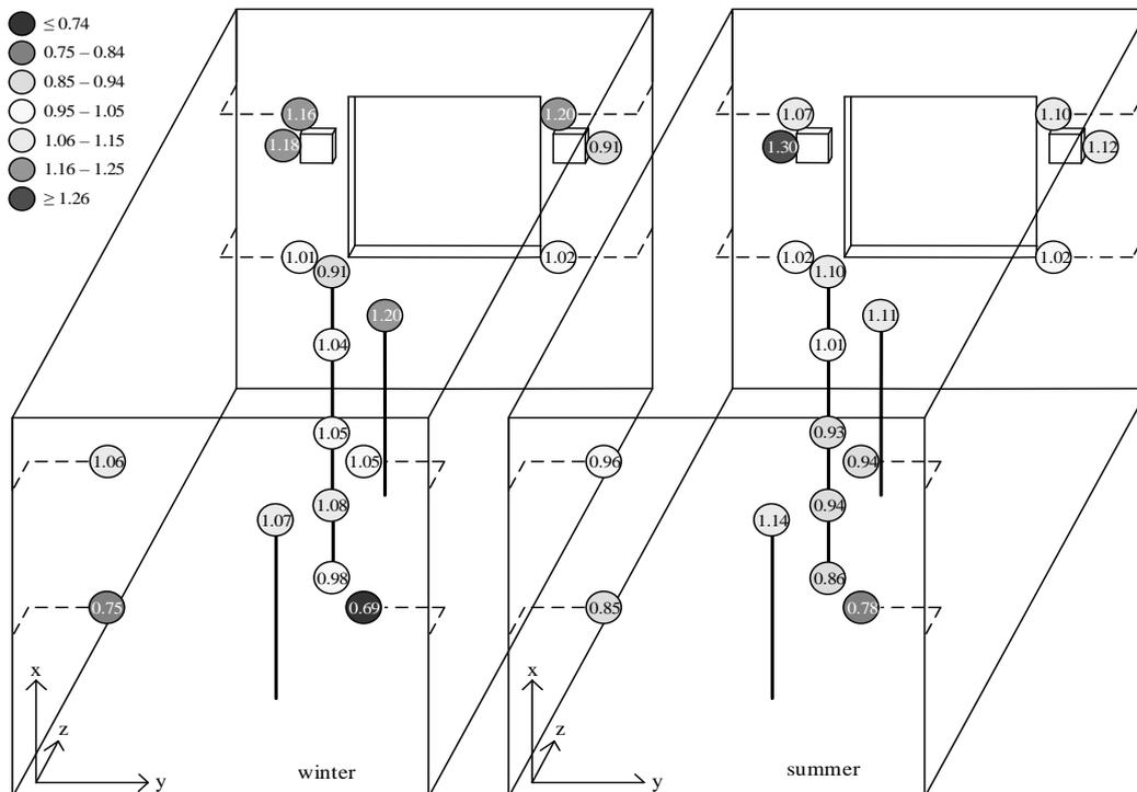
**Figure 1.** Local air exchange indices  $\epsilon_{N,j}^a$  (2-3) at  $\dot{V} = 15 \text{ m}^3 \cdot \text{h}^{-1}$  at winter (left) and summer (right) supply air conditions as well as isothermal supply air conditions
