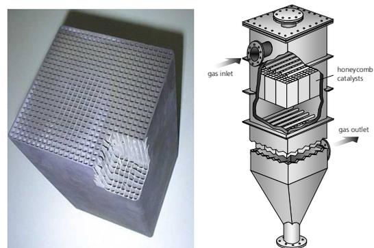
**Figure 1:** Catalytic monolith (left) and tar reformer with two layers of monoliths (right)
