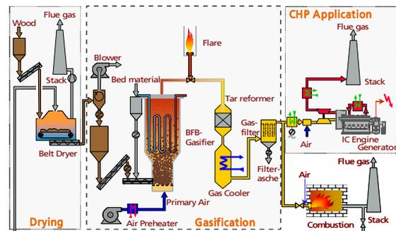
**Figure 2:** Power plant concept based on bubbling fluidized bed gasification and dry gas cleaning
