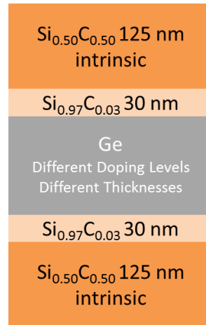
Figure 1: Structure of Ge lifetime samples for all irradiations with passivation and mirror layers on both sides. Ge wafers with different doping levels and thicknesses were used.
