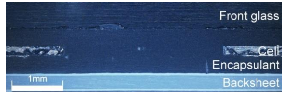
Figure 4: Microscope image showing an example of a module cross section with a 3 mm cell gap.
