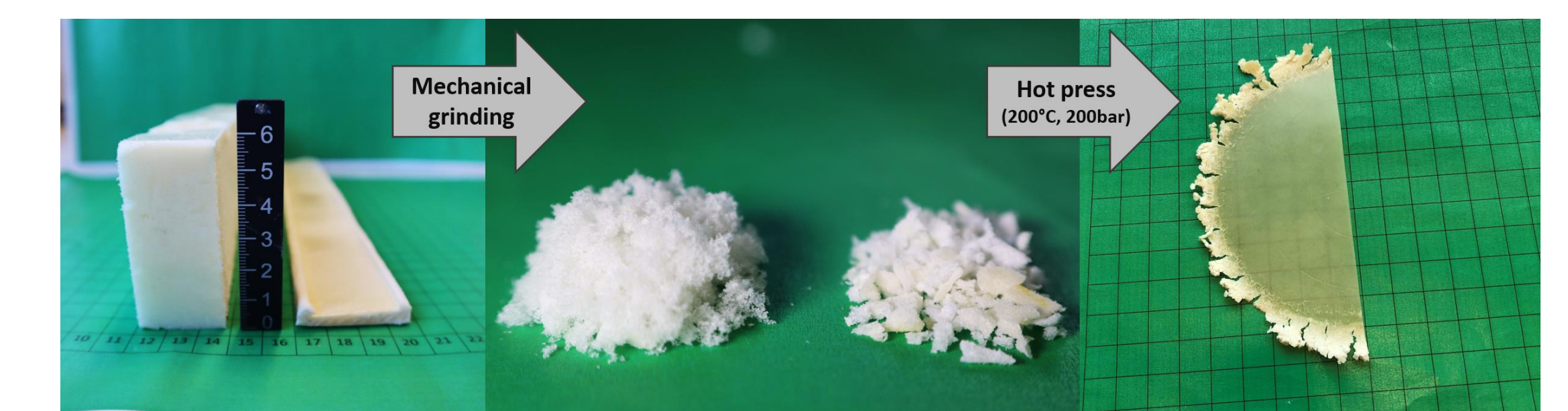
Figure 5 – Recycling/Reuse of linear SMP-PU foams → foam in original (left, left) and compressed state (left, right), ground foam (center) and recycled film (right).
