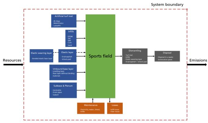
Figure 35: System boundaries of the artificial sport pitch
