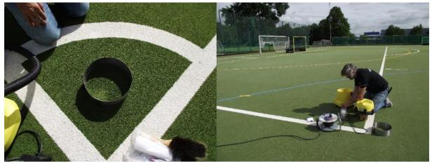
Figure 47: Sampling body at corner point (I.); sampling with vacuum cleaner (r.)
