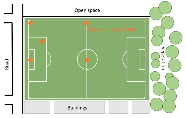
Figure 17: Location of the measuring points within a pitch quarter
