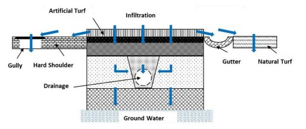
Figure 5: Possibilities of drainage for artificial turf pitches
