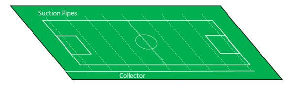
Figure 7: Drainage system for artificial turf pitches
