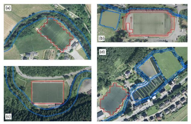
Figure 14: Examples of artificial turf pitches located close to surface waters. Artificial turf pitch in red, nearby surface waters in blue.<sup>41</sup>
