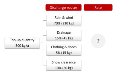
Figure 32: Mass balance on the consumption and transfer of infill for artificial turf pitches in Germany
