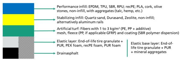
Figure 2: Schematic presentation of the layer-by-layer structure of artificial turf pitches
