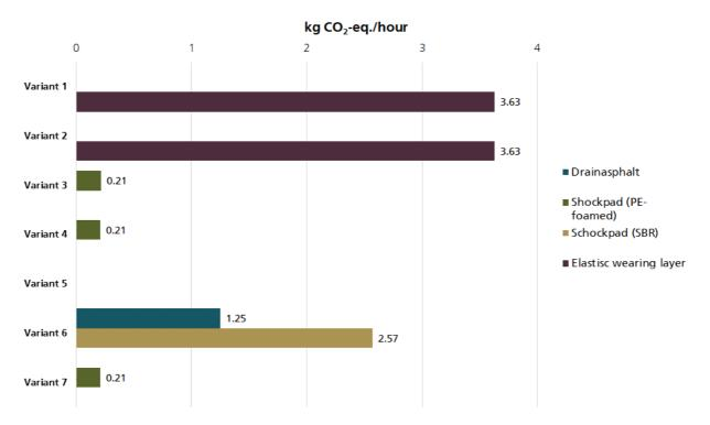
Figure 38: Comparison of the greenhouse gas emissions of various damping layers from the manufacturing phase
