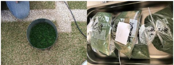
Figure 48: Sampling point after sampling (I.); packaged infill samples before fractioning (r.)
