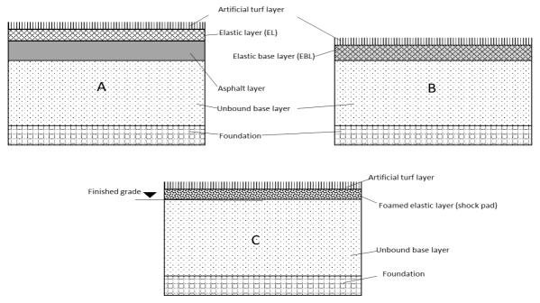
Figure 1: Structure of an artificial turf pitch, construction method A and B, in accordance with DIN 18035-7, and construction method C with finished grade (authors' diagram)
