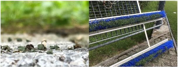
Figure 51: Performance infill next to the pitch (I.); grid with brush (r.)
