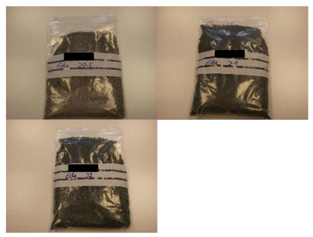
Figure 46: Infill samples fractionated via sieve analysis
