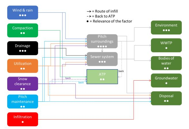
Figure 33: Transfer routes and fates of infill, schematic diagram [Fraunhofer UMSICHT]
