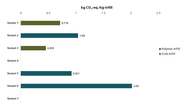
Figure 39: Comparison of the greenhouse gas emissions of various infill versions from the manufacturing phase
