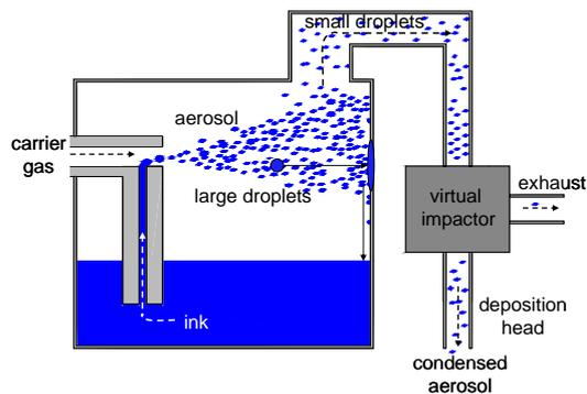
Figure 2: Working principle of the pneumatic atomizer including the virtual impactor. Only smaller droplets are transported by the carrier gas whereas larger droplets remain in the ink jar.
