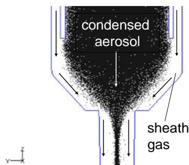
Figure 3: Simulation of the gas flow in the deposition head. A droplet size of  $d_{\text{drop}} = 1 \mu\text{m}$  an  $N_2$  as process gas was assumed.
