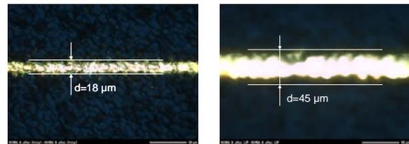
Figure 4: Aerosol printed finger width of  $d = 18 \mu\text{m}$ , after firing (left) and  $d = 45 \mu\text{m}$  after LIP (right)
