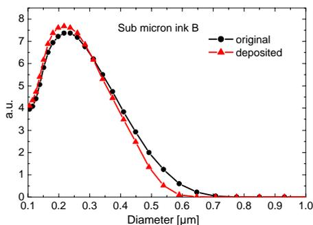
Figure 6: Particle size distribution of a paste suitable for aerosol printing. The distribution is constant – no separation in small and large particles is taking place during printing process.
