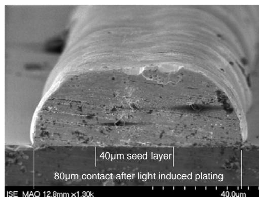
Figure 1: Cross section of an aerosol printed, fired and plated contact finger. About 20  $\mu\text{m}$  of silver is plated on top of the seed layer. The height of the seed layer is about 1.5  $\mu\text{m}$ .
