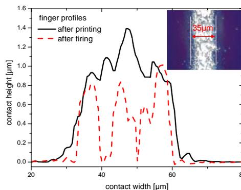
Figure 7: Cross section of a printed (solid line) and fired contact (dashed line). The small picture shows a top view of an aerosol printed and fired contact.
