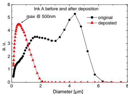
Figure 5: Particle size distribution of a conventional screen-print paste. The size distribution after printing is shifted towards particle sizes below 2  $\mu\text{m}$ .
