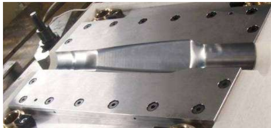
Shell with die shape (front side)
