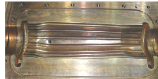
Basic body with cooling channels
