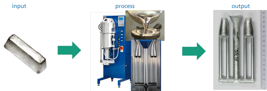
Figure 2. Schematic representation of the permanent mold casting process including the ingot as input and the cast part as output.
