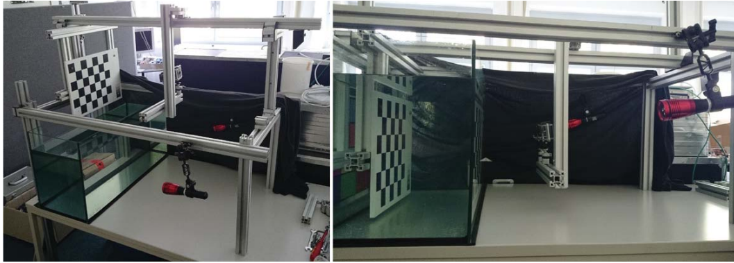
Fig. 6. Generation of ground truth data. A checker target that is fixed to the stereo camera system can be lowered into water.
