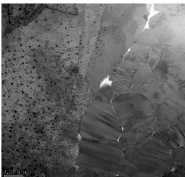
Figure 4: Phase boundary between steel (left) with precipitations (dark spots) and ceramic. Note the region free of precipitations near the phase boundary.
