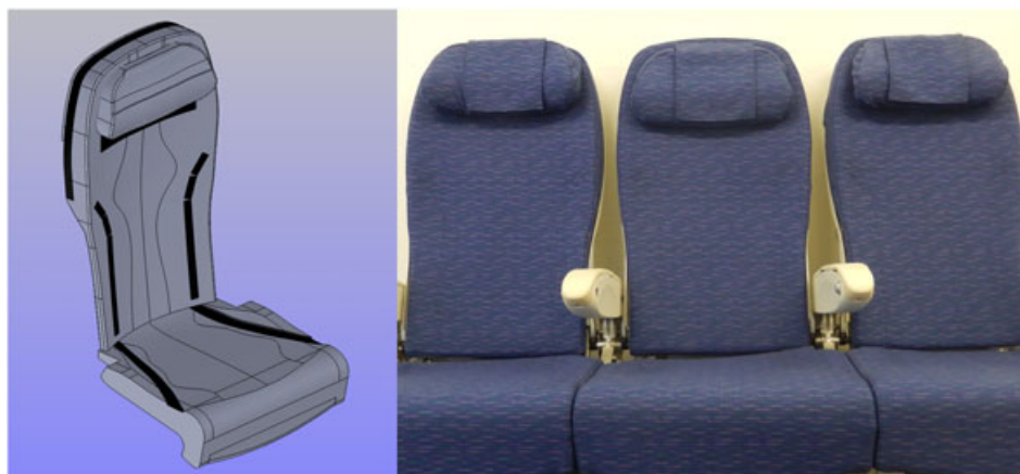
FIGURE 1 Aircraft seating cushions: schematic diagram (left) and aircraft seat demonstrator “green PUR seating cushion” (right) [Colour figure can be viewed at wileyonlinelibrary.com ]
