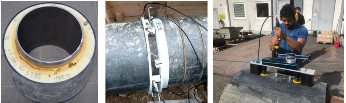
Figure 2. Different methods to measure the adhesion between steel pipe, PUR and PE-casing: In the laboratory (left picture, source FFI Hannover) and the field (middle, source: IMA Dresden) and (right picture, source: RISE)
