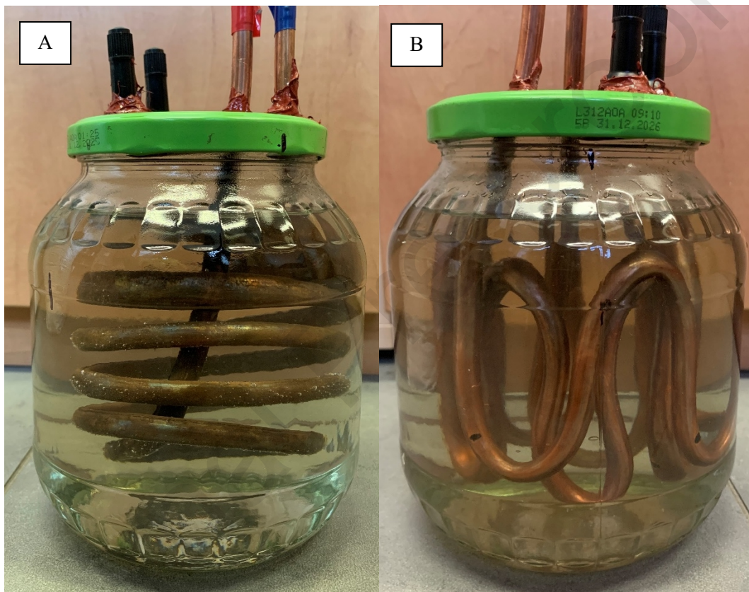
187 188 Fig. 1. Test module heat exchangers: A Spiral, B Toroid squiggle.
