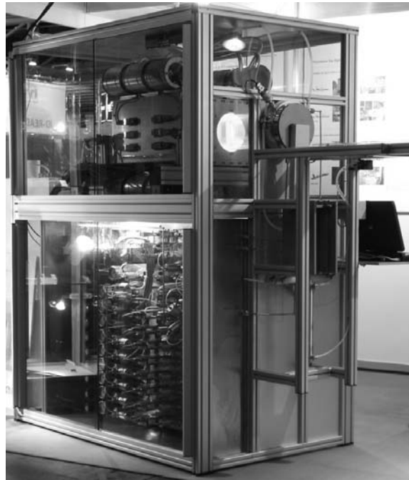
Fig. 1: Front view of the RTCVD160 system. In the lower part the gas system is visible. The upper part houses the optically heated furnace and the reactor tube.
