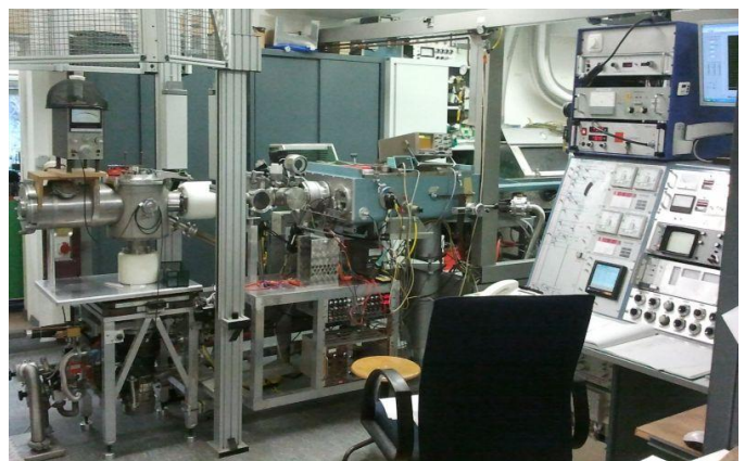
Fig. 1 The isotope separator at the University Bonn used for proton irradiation. The samples were placed in a vacuum chamber.
