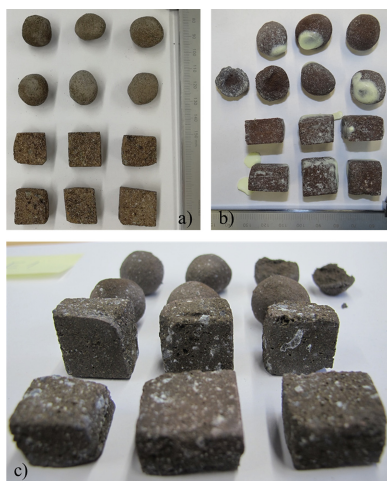
Fig. 3. Optical modification of fillers cycled with solar salt, a) before in contact with salt, b) after sampling, c) after separation of salt in oven
