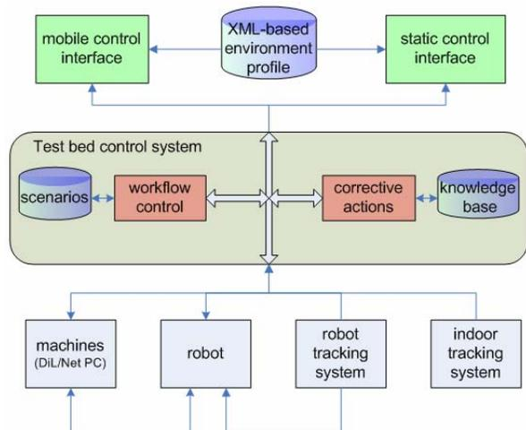
**Figure 3. The structure of the test bed software**
