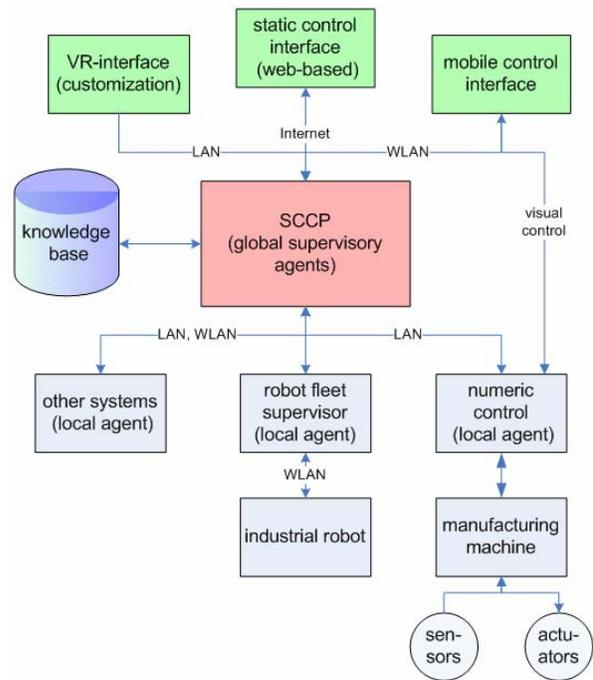
Figure 1. The architecture of the SCCP
