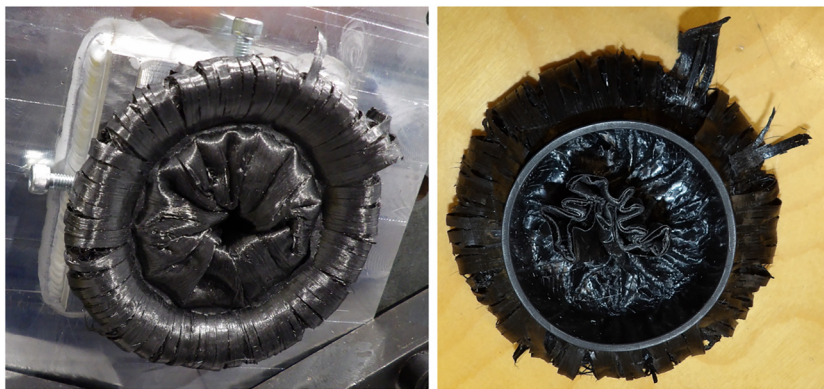
Figure 9: Example fracture images of crash box No. 04: Trigger side (left); Flat side (right).
