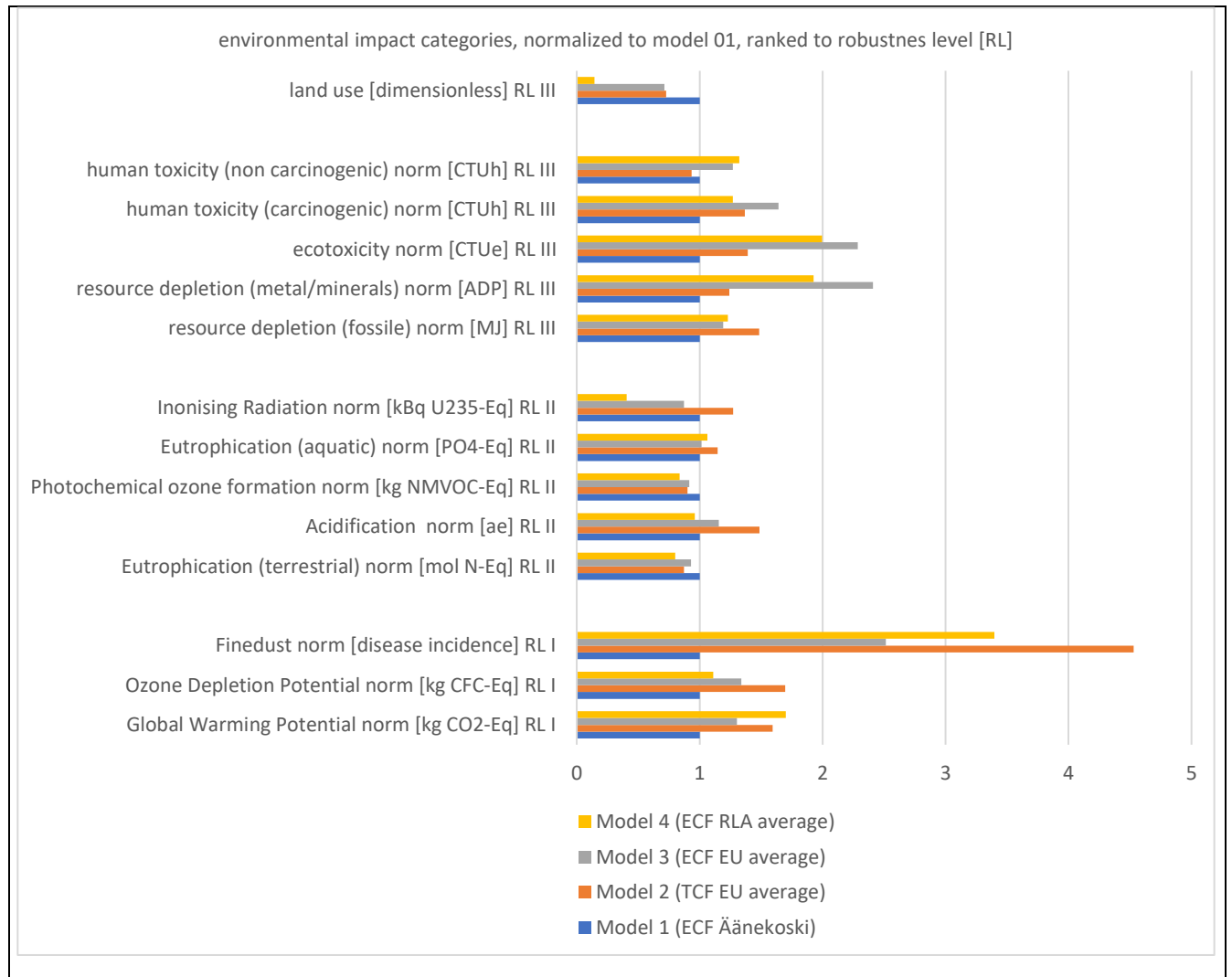
Figure 07: Environmental Impact, with (RL) robustness level I (GWP, Particulate Matter, Ozone Depletion Potential), and RL II (Eutrophication terrestrial, Acidification, Photochemical Ozone Formation, Eutrophication aquatic, Ionising radiation), and III (resource depletion fossil, resource depletion metal/minerals, ecotoxicity, human toxicity carcinogenic, human toxicity non carcinogenic, land use), is shown normalized to model 01 (ECF Äänekoski).
